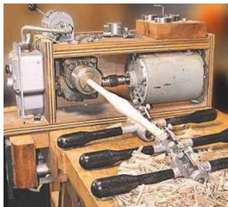
▲ Pic. 3 Jeff's 'turning engine' and the rotary planes used to rough out the spindles
